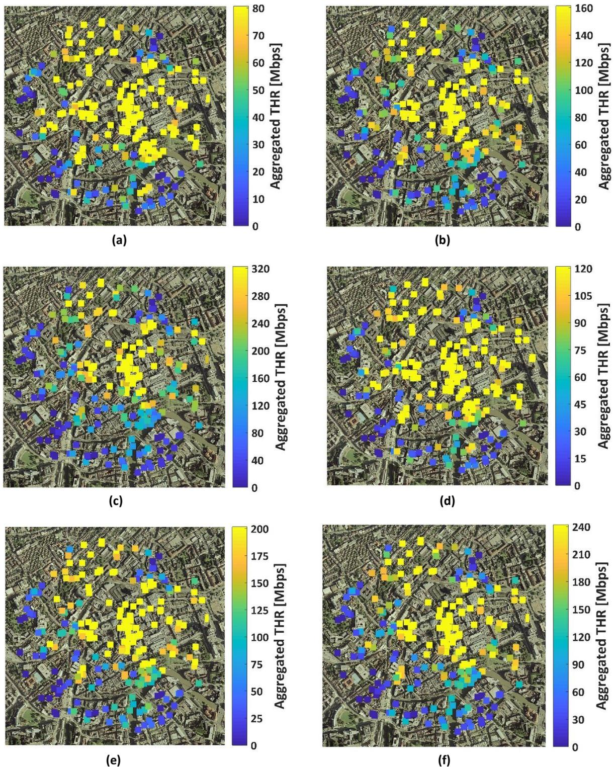
Fig. 5 Achieved aggregated THR coverage map for different CA scenarios in the city center of Bristol: a) CA 1-1; b) CA 2-2; c) CA 4-4; d) CA 2-1; e) CA 4-1; f) CA 4-2.
