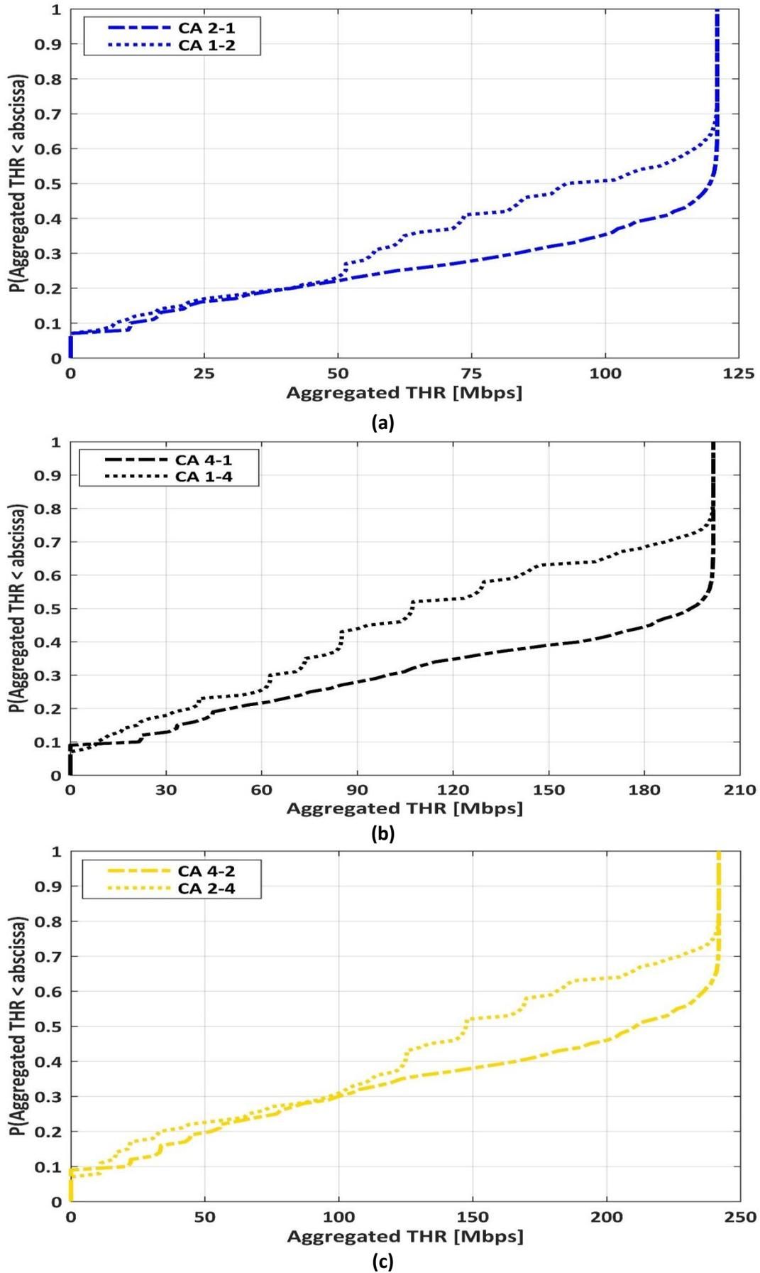
Fig. 2. CDF of UEs aggregated THR for CA scenarios with same number of aggregated spatial streams: a) three aggregated spatial streams; b) five aggregated spatial streams; c) six aggregated spatial streams.
