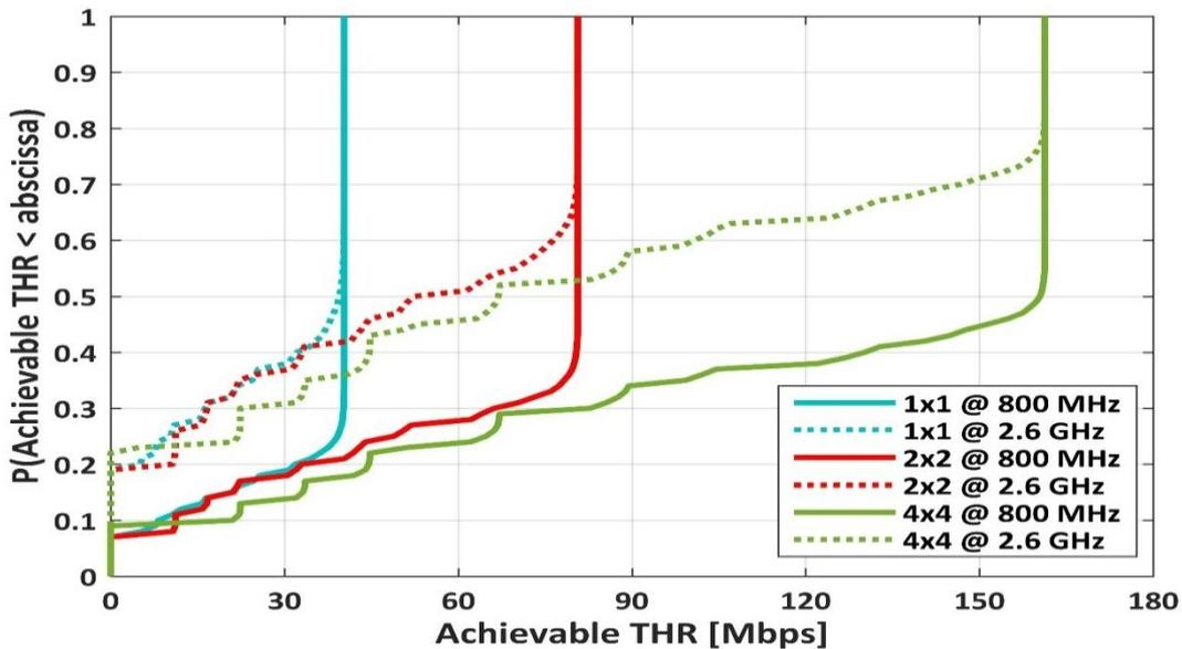
Fig. 1. CDF of UEs THR for individual CCs and antenna systems.
